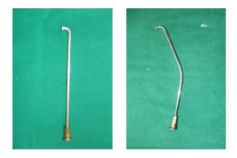
Figure 4: Straight And Bent Motorcycle Spoke
