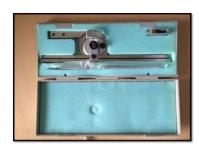
Fig 1: Bevel protractor for Buccolingual measurement
