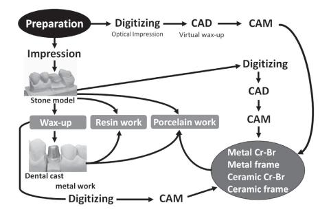
Fig-2. An overview of current dental CAD/CAM Fig. systems using for the fabrication of crown-bridge restorations
